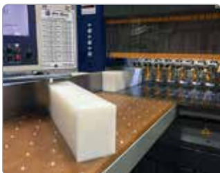
Panel Saw Cutting
