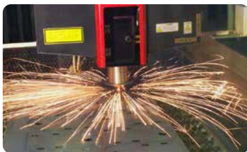
Laser cutting available for plate up to 3/8" thick. Plasma cutting plate from >1/2" thick up to 1" thick.
