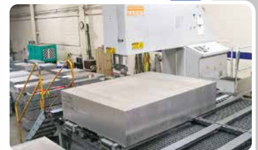
Precision sawing of aluminum mold plate up to 30" thick.
