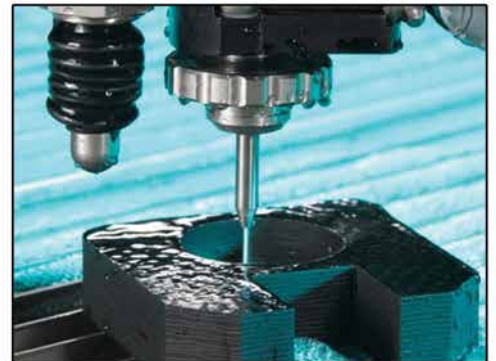
Tough materials, capable of cutting fiberglass, glass-filled, rubber, urethane and foam parts.
