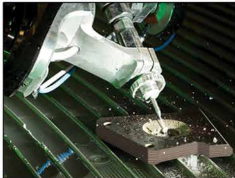
5-Axis technology, we are able to produce parts quicker, more accurate bevels and do 3D cutting.
