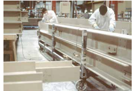
Prefabrication of support beams can include bonding predrilled angles and plate for connections.
