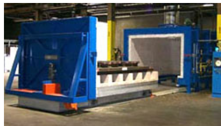
Our furnace is 96" wide x 144" long x 54" high with a weight capacity of 30,000 lbs.
