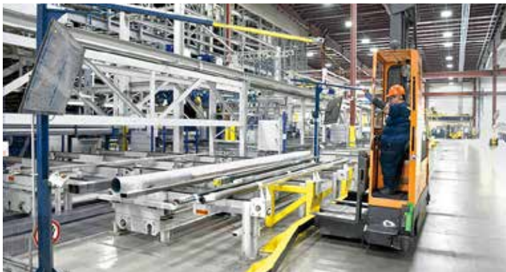
Transporting material from Automated Storage & Retrieval System (ASRS)
