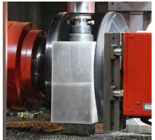
Super Square precision 2, 4, 6 side milling
