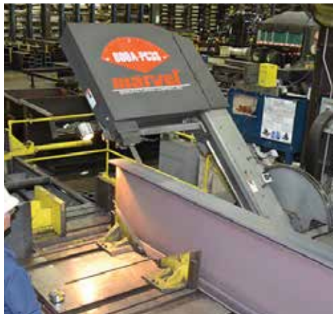
Miter cutting a steel beam
