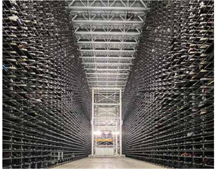
Automated Storage & Retrieval System (ASRS) in Potterville
