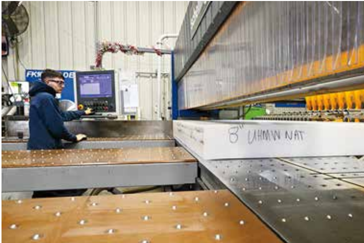
8" thick UHMW plastic sheet cut on a panel saw
