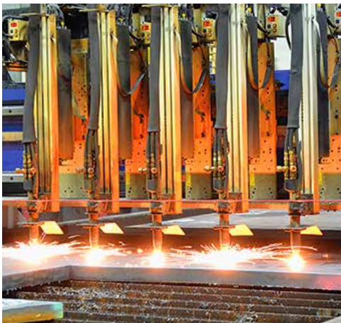
Multi-head oxy-fuel cutting
