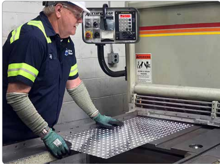
Our shears have a maximum plate capacity of 1/2" thick x 144" x 144"
