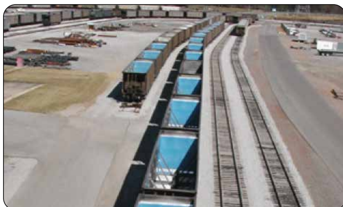
Rail cars lined with TIVAR® 88-2 prevent sticking of sub-bituminous and ignite coals
