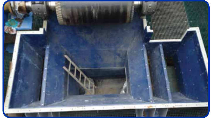
TIVAR® 88-2 lined receiving hopper provides reliable bulk material flow
