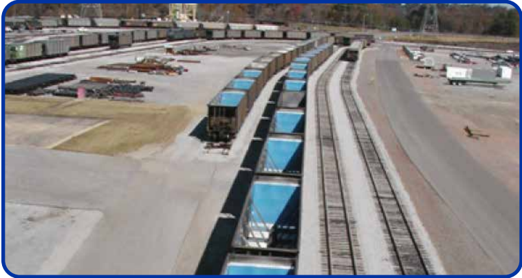
Rail cars lined with TIVAR® 88-2 prevent sticking of sub-bituminous and ignite coals
