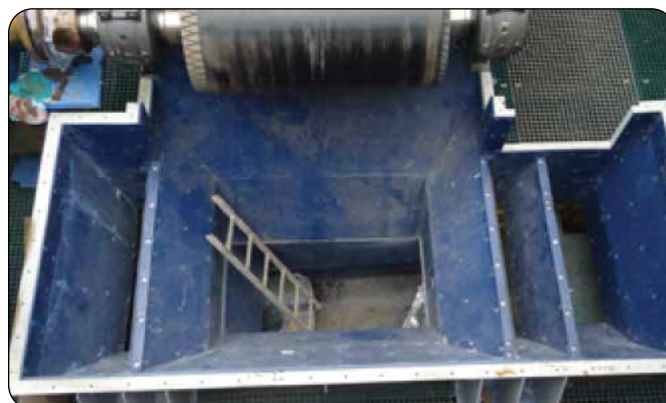
TIVAR® 88-2 lined receiving hopper provides reliable bulk material flow
