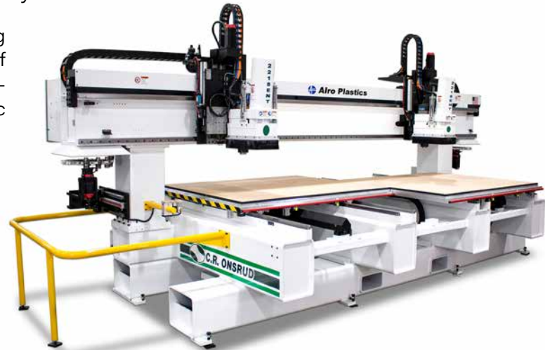
Pictured, twin table CNC router with dual heads and automatic tool changers
