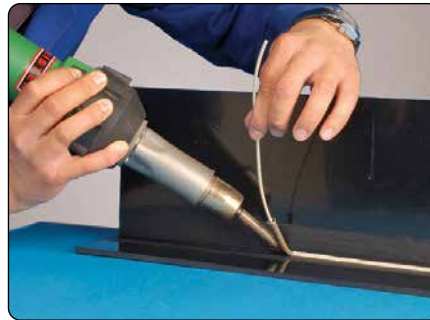
Pictured, a modified extrusion welder being used to weld a custom container
