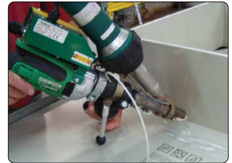
Pictured, a modified extrusion welder being used to weld a custom container
