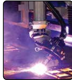
Our HPR 400 plasma cutting machine with bevel cutting capabilities.
