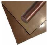
Delrin® 570 GF20 glass-filled stock shapes exhibit the basic Delrin® properties plus high strength. Overall mechanical properties and dimensional stability are enhanced in this tough material. Specific property advantages include increased stiffness, better creep resistance and a higher dimensional stability. Parts designed using glass-filled will exhibit high fatigue endurance, low deformation under load and good impact resistance.
