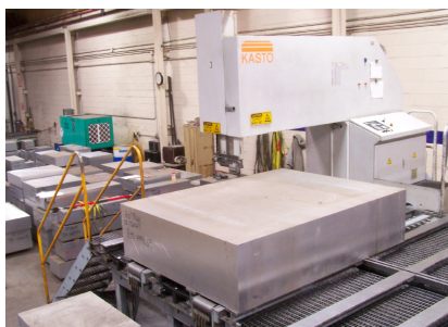
Precision sawing mold plate up to 30" thick.
