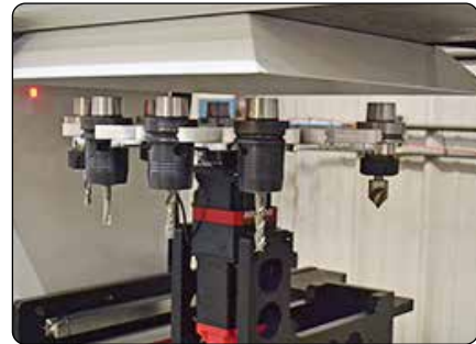
Pictured, twin table CNC router with dual heads and automatic tool changers
