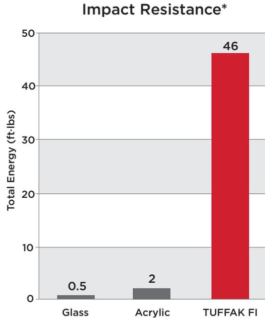
\*Instrumented Impact per ASTM D 3763,
