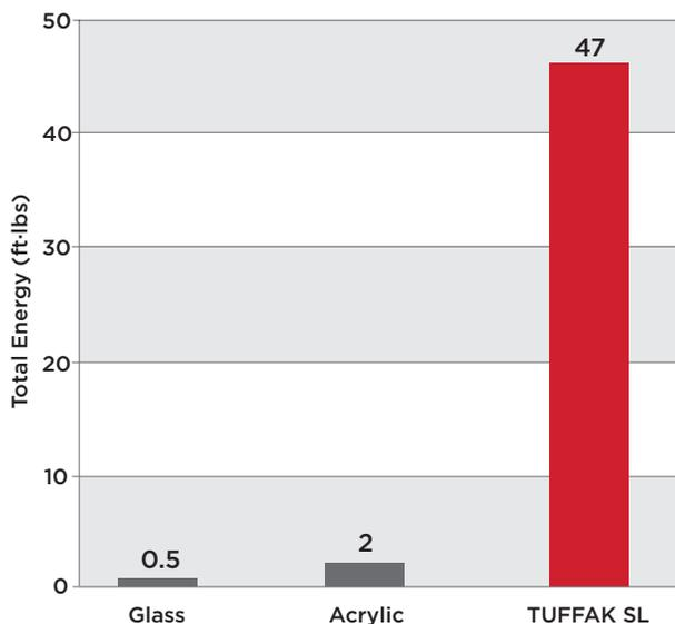
\*Instrumented Impact per ASTM D 3763, sample thickness 0.125" nominal
