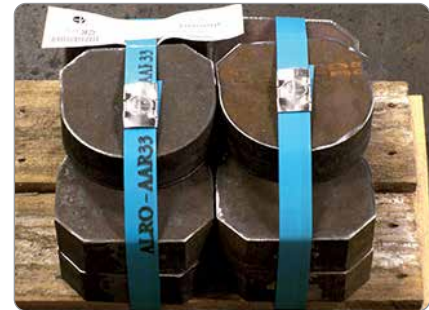
Edges ground on all flame cut pieces to deburr them for safer handling.
